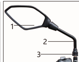
The fastening torque for nut 3:40Nm
